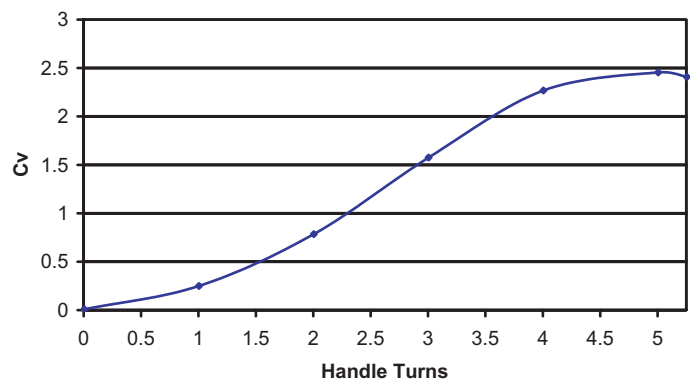
Cv vs Handle Turns for a 5E Throttle Valve with 1/4" Orifice
